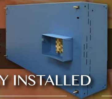
Back of IR heater panels include threaded studs for mounting, and a junction box with knockouts for service connection to a hi-temp ceramic terminal block.
